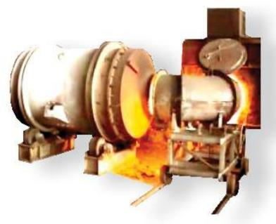
The furnace consists of a cylindrical shell fitted with two steel tyres supported on rollers mounted on a fabricated steel frame. The shell has two spouts and two lifting trunions and is rotated by friction between the tyre and rollers, which are driven by a motor via a worm reduction gear. Manual drive provision is also a standard feature.
